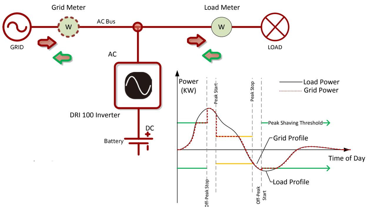
Figure 1: Simplified circuit diagram of a Peak Shaving application
