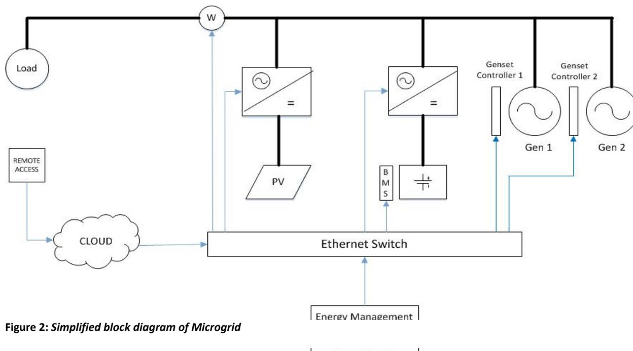
Figure 2: Simplified block diagram of Microgrid
